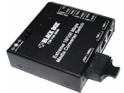
The front side of the unit has two twisted-pair 10/100Mb switch ports and one 10 or 100Mb fiber port. Both the RJ-45 ports of the LBH100A and LBH110A Series Media Converter Switches support auto-cross (MDIX) operation performing the auto-cross function under auto-negotiation mode only. The 10Mb fiber (LBH110 models) are factory configured at Half-duplex, and 100Mb (LBH100 models) are factory configured at Full-Duplex.
