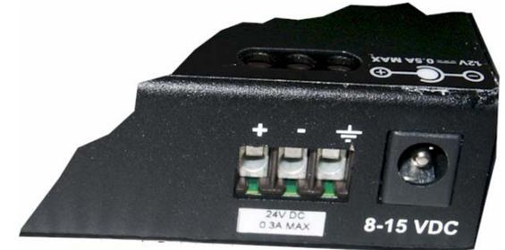
The connection procedure is straightforward. Simply insert the DC leads to the LBH100H's power terminals, positive (+) and negative (-) screws. The use of Ground (GND) optional; it connects to the LBH100H chassis. Ensure that each lead is securely tightened from the top, as shown here.
