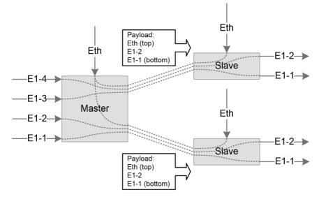
Figure 3.7 Automatic configuration Star-topology
