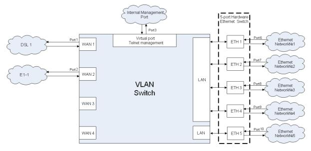
Figure 3.11 Internal Switch for single-channel devices (SA-RC-ETHERLINK\_IVL-2E1B/4Eth-RP,V90)
