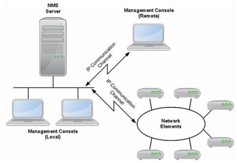
Figure 3.25 The structure of SNMP-based NMS.
