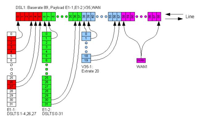
Figure 3.12 Example of distribution of time slots in an SHDSL frame at a line rate of 89x64 Kbit/s in the mode when both E1 interfaces and both internal WAN1 and WAN2 ports are used for the termination device.
