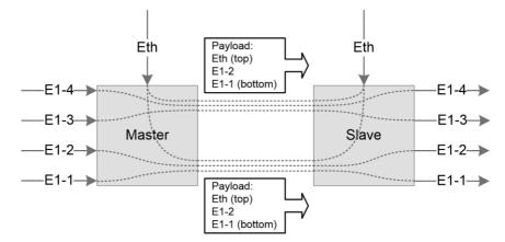
Figure. 3.8 Automatic configuration 2x E1 and Ethernet are transmitted over two SHDSL link.
