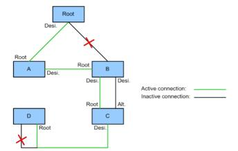
Figure 3.15 Change of Port role upon network failure.
