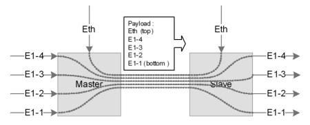
Figure. 3.6 Automatic configuration, 4x E1 and Ethernet are transmitted over one SHDSL link
