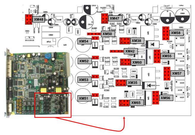
Figure 3.1 Remote power jumper location
