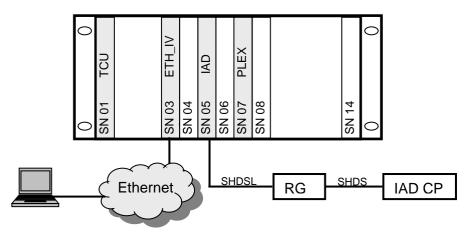
Figure 3.20 Example of Telnet access through Etherlink IV LTU in subrack
