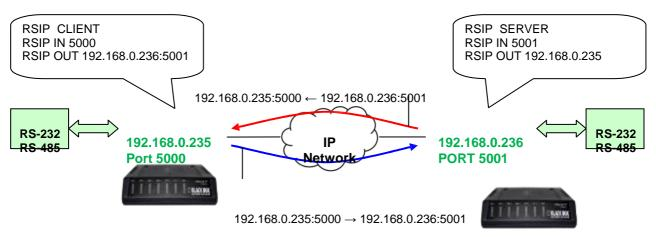
Picture 2.4. Serial Data Transmission with TCP Point-To-Point
