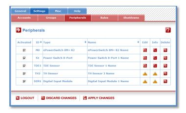
The Peripherals page is used to configure all peripherals connected to the Power Switch Master.
