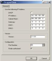
This page enables to define all IP parameters of the Power Switch Master device and displays the version of the Firmware. The Finder program is authorized at factory settings.
