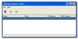
3. Open the File menu and choose **CONFIGURE** (or click on the second left button in the tool bar) to configure the network parameters.
