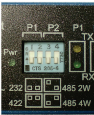
Figure 5-7. DIP Switches on the ICD120A.
